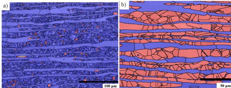
Fig6. EBSD phase map of a) mechanically polished sample and b) electropolished sample (blue=bcc, red=fcc)<sup>9</sup>.
