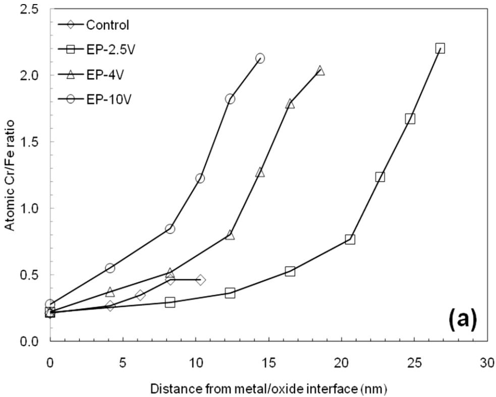
Fig4. (a) Cr/Fe atomic ratio for naturally grown passive film on 316L-SS (control), and passive films formed on 316L-SS by electrochemical polishing at cell voltages of 2.5, 4 and 10 V.<sup>5</sup>
