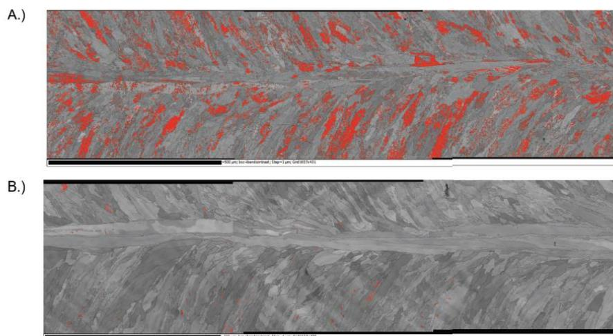
Fig7. Band contrast map of plan view section of weld metal. Red pixels denot phase indexed 'bcc' ferrite for A.) mechanically polished and B.) electropolished material<sup>10</sup>
