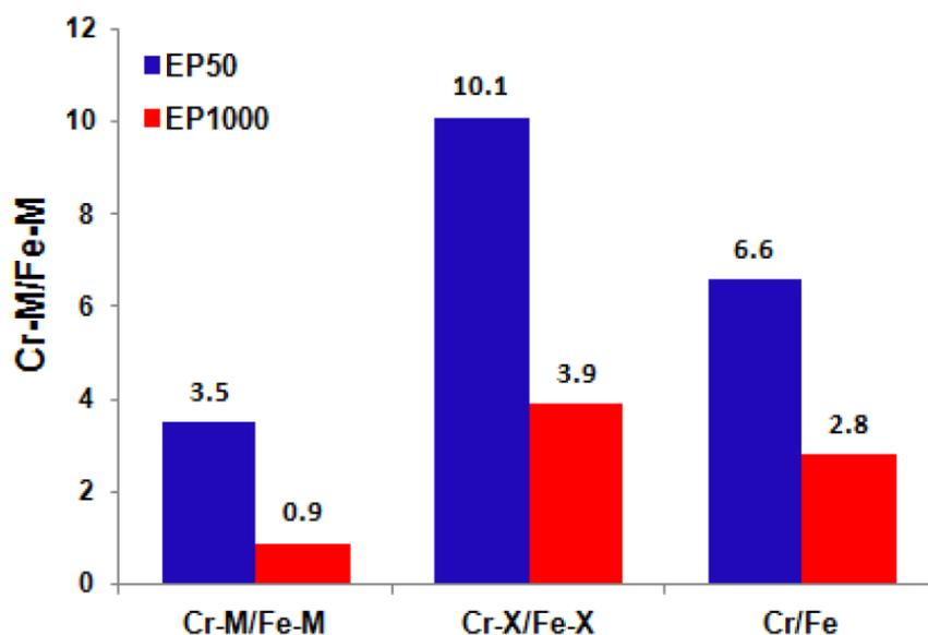
Fig2. Chromium metal to iron metal (Cr-M/Fe-M), chromium compounds to iron compounds (Cr-X/Fe-X) and total chromium to total iron (Cr/Fe) ratios as obtained on the basis of high-resolution XPS spectra<sup>2</sup>
